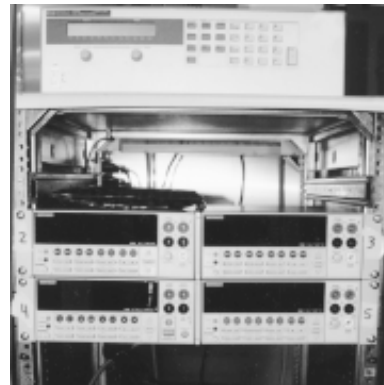
(Left) Some of the equipment being used in the Power!Lab: the HP Power Supply (top), three Keithley benchtop multimeters and a Keithley sourcemeter. (Photo by Jose Alvarez)
