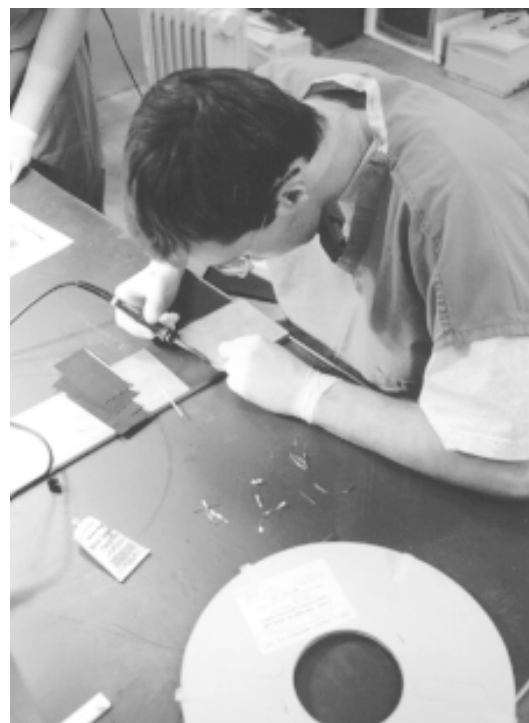
Left: Chris Deline is soldering cells cut by Spectrolab before they become the part of the array.
